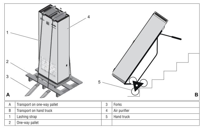
Use a forklift or pallet truck to transport the air purifier on its one-way pallet (A).
