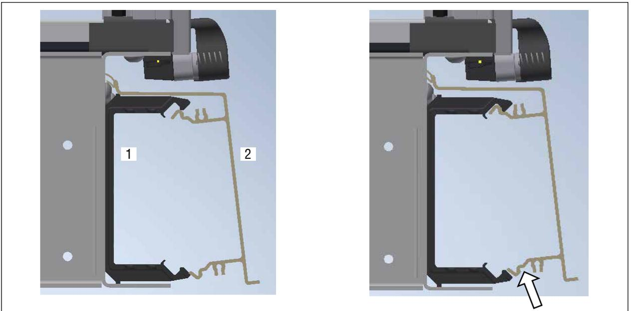
Fig. 32 Threading on the upper nose of the cable duct clamp
