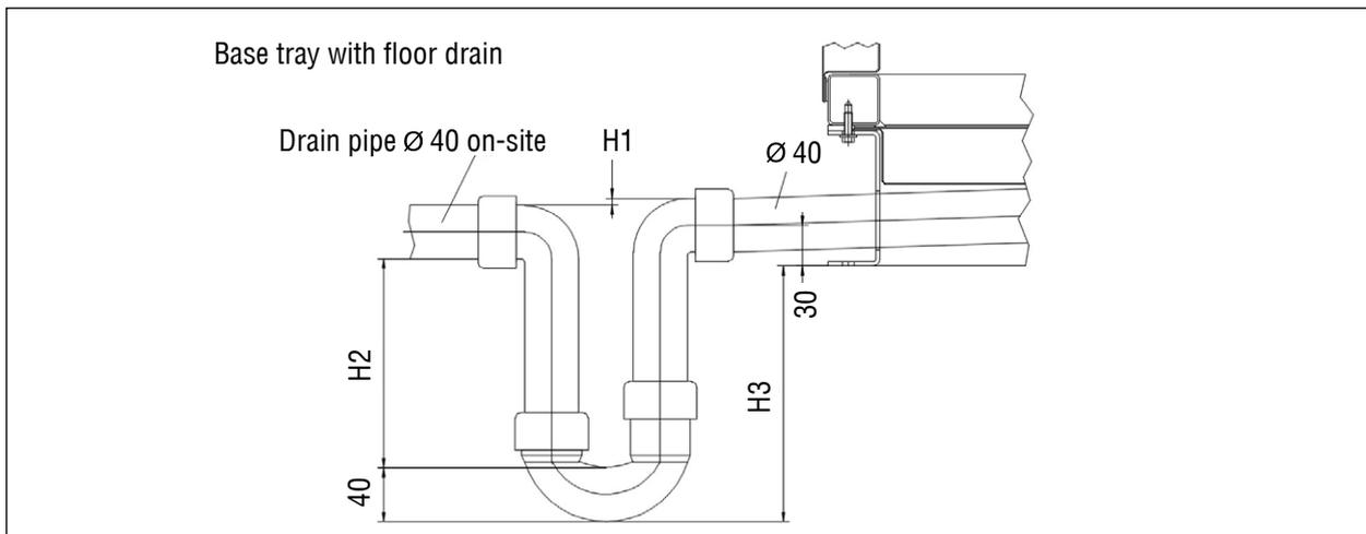
Fig. 44 Connection of the condensate drain with snake siphon
