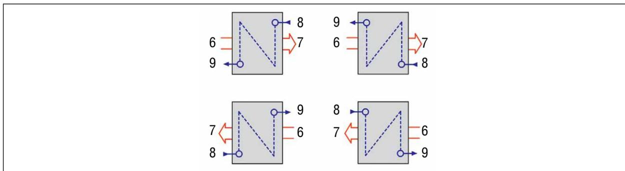
Fig. 41 Counterflow principle for heat exchanger connection
