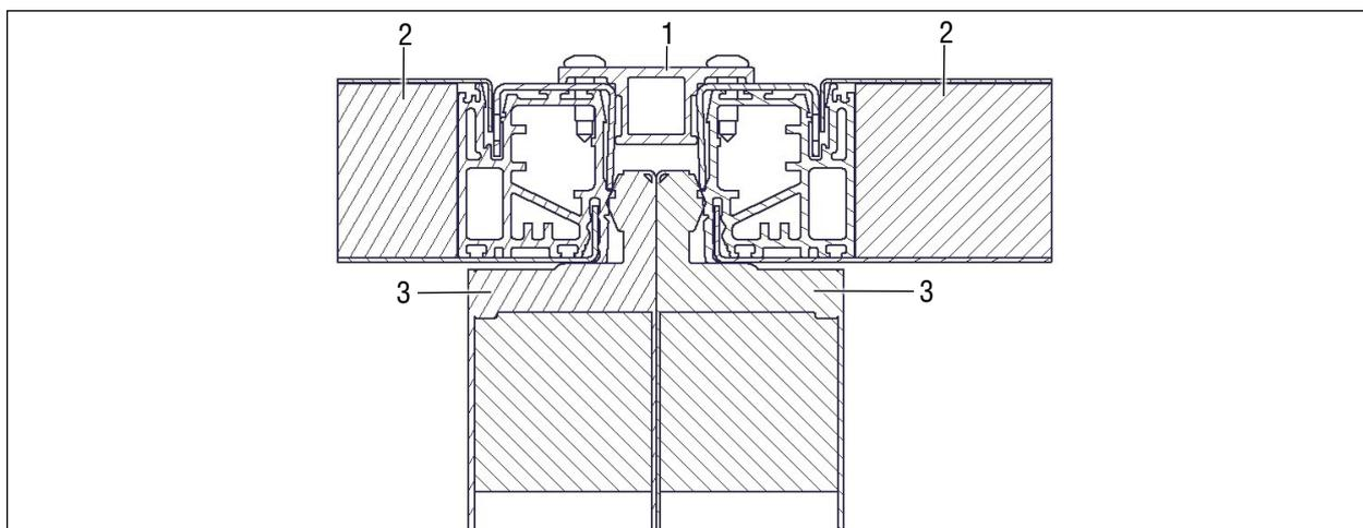
Fig. 16 Unit arrangement next to one another without mixing chamber
