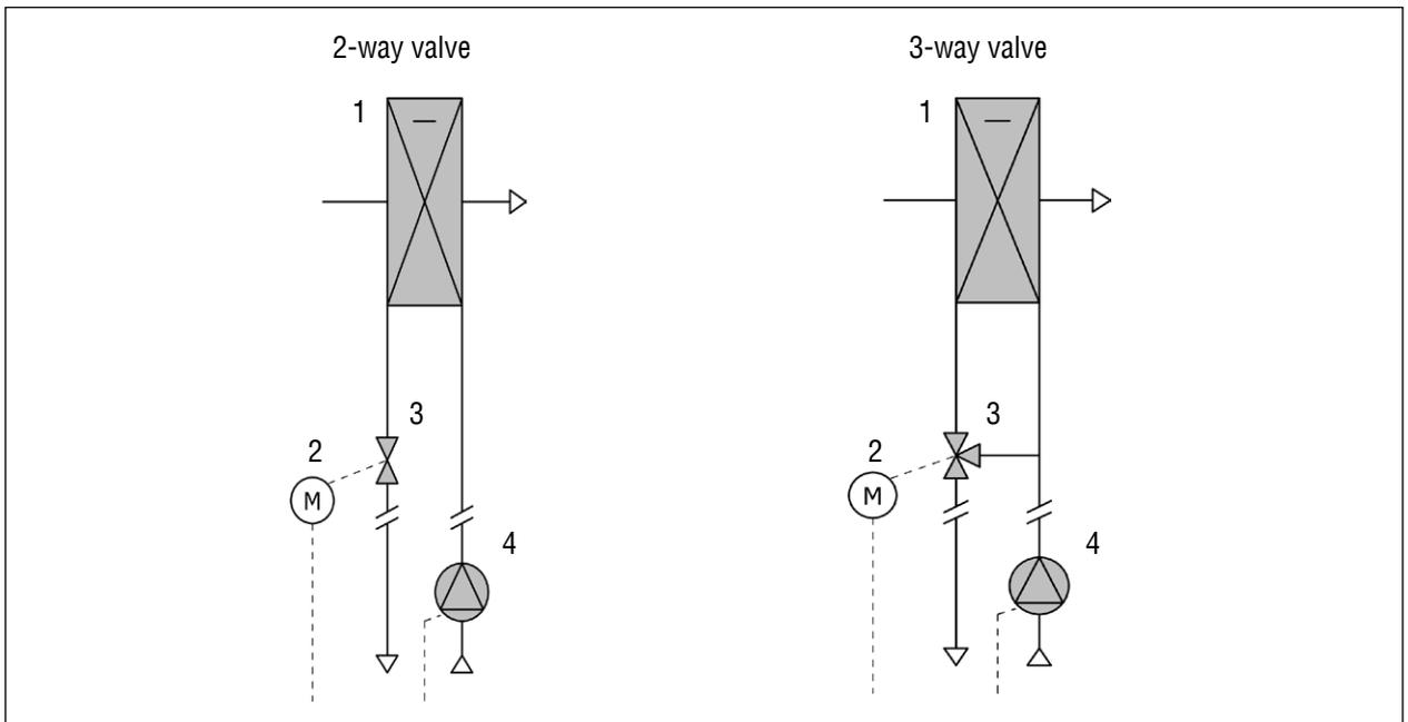
Fig. 40 2-way valve and 3-way valve connection versions
