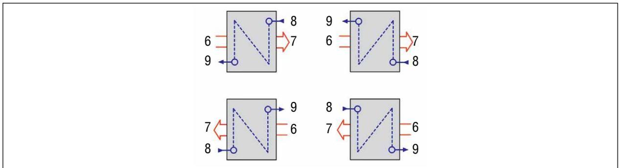
Fig. 37 Counterflow principle for heat exchanger connection
