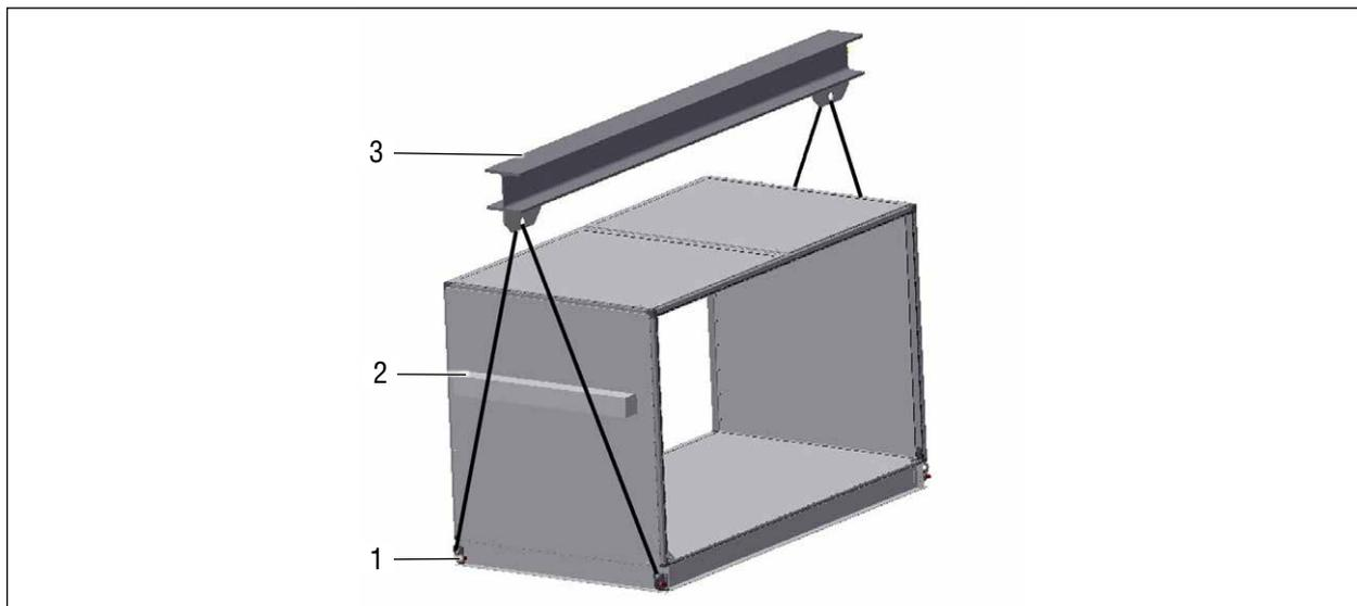
Fig. 3 Transport using a base frame bracket
