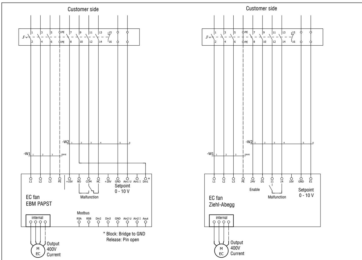
Fig. 53 Connection of EC fans from EBM Papst (left) or Ziehl-Abegg (right)
