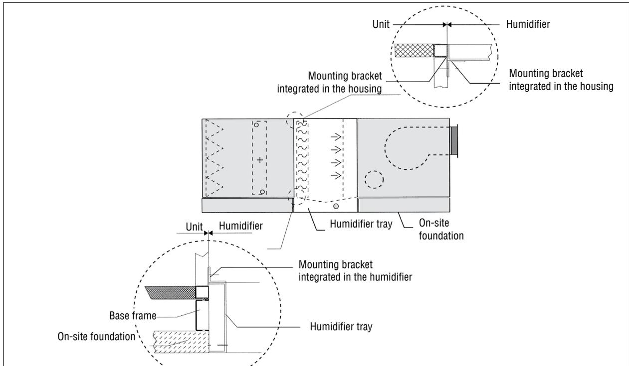
Fig. 19 Unit arrangement next to one another with humidifier
