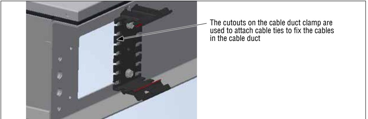
Fig. 31 Detail of cable duct clamp
