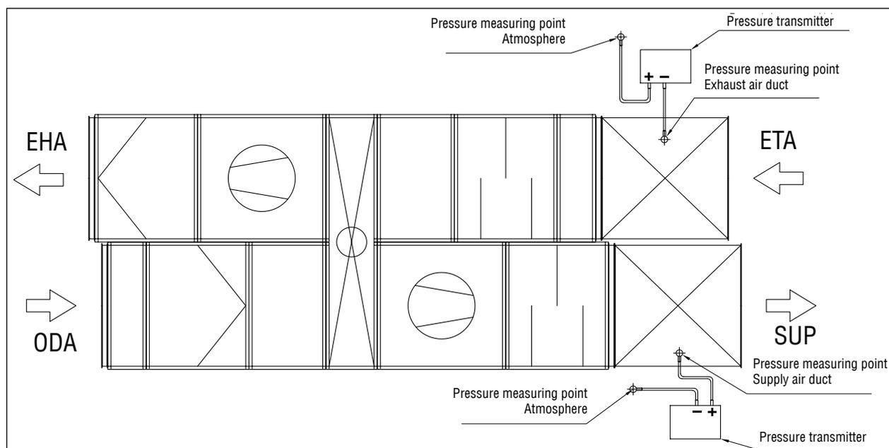
Fig. 64 Wiring diagram for volume flow measurement
