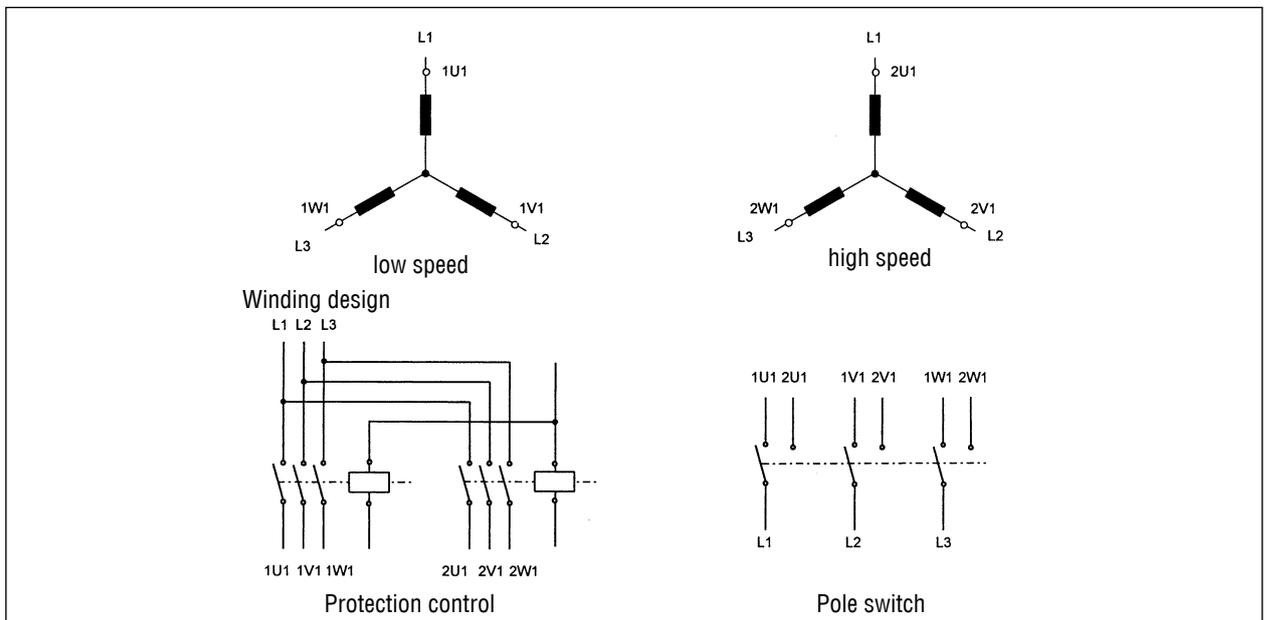
Fig. 49 Circuit of three-phase motors for two speeds
