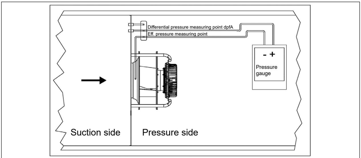
Fig. 62 Wiring diagram for volume flow measurement
