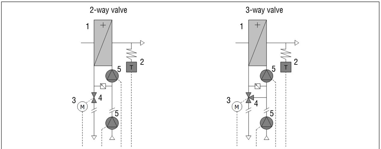
Fig. 36 2-way valve and 3-way valve connection versions
