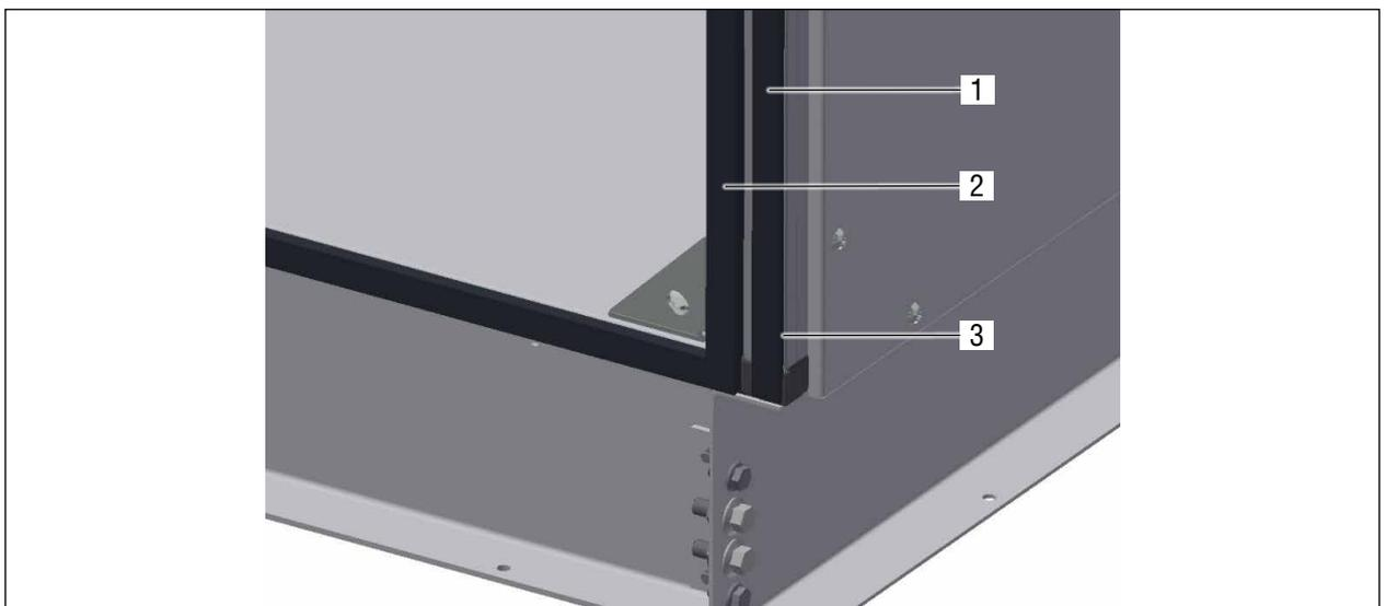
Fig. 8 Separation point sealing with outdoor installation
