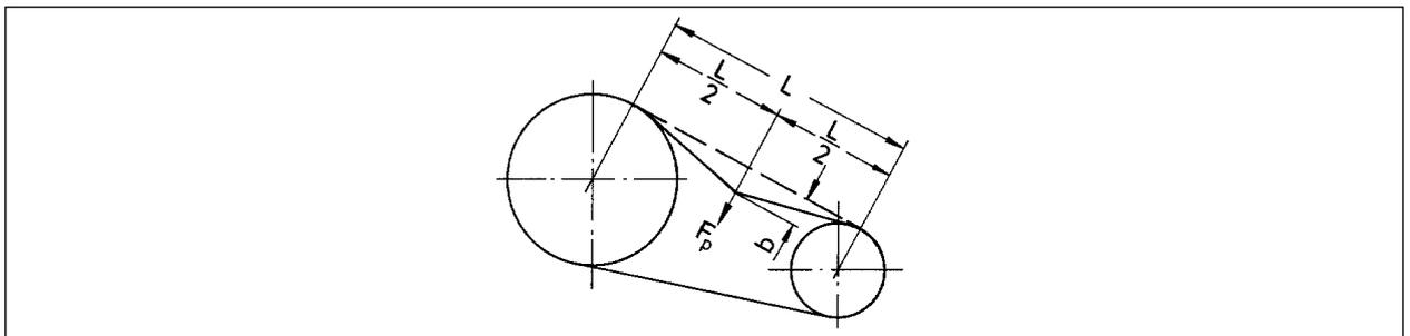
Fig. 59 Checking the belt tension on the V-belt drive
