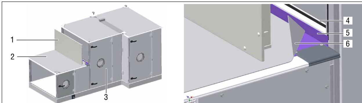
Fig. 25 Weatherproof units with height offset
