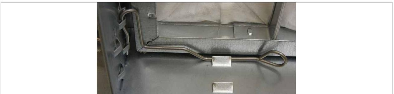
Fig. 68 Filter mounting frame, left filter clamp
