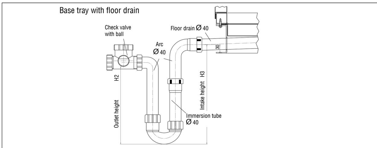
Fig. 45 Connection of the condensate drain with ball siphon with overpressure
