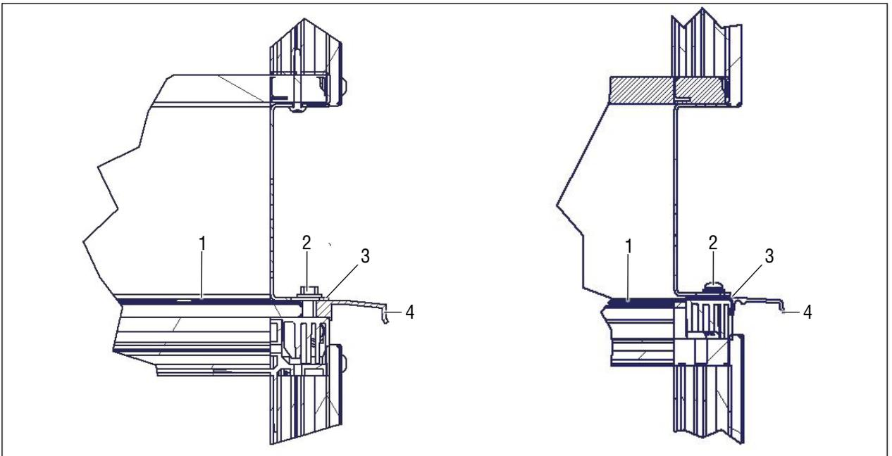
Fig. 12 Unit arrangement roof assembly with unit frame profile (left) and without unit frame profile (right)
