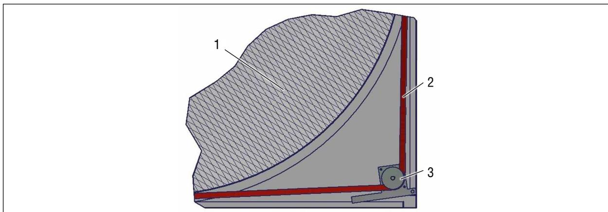
Fig. 57 Drive V-belt installation situation
