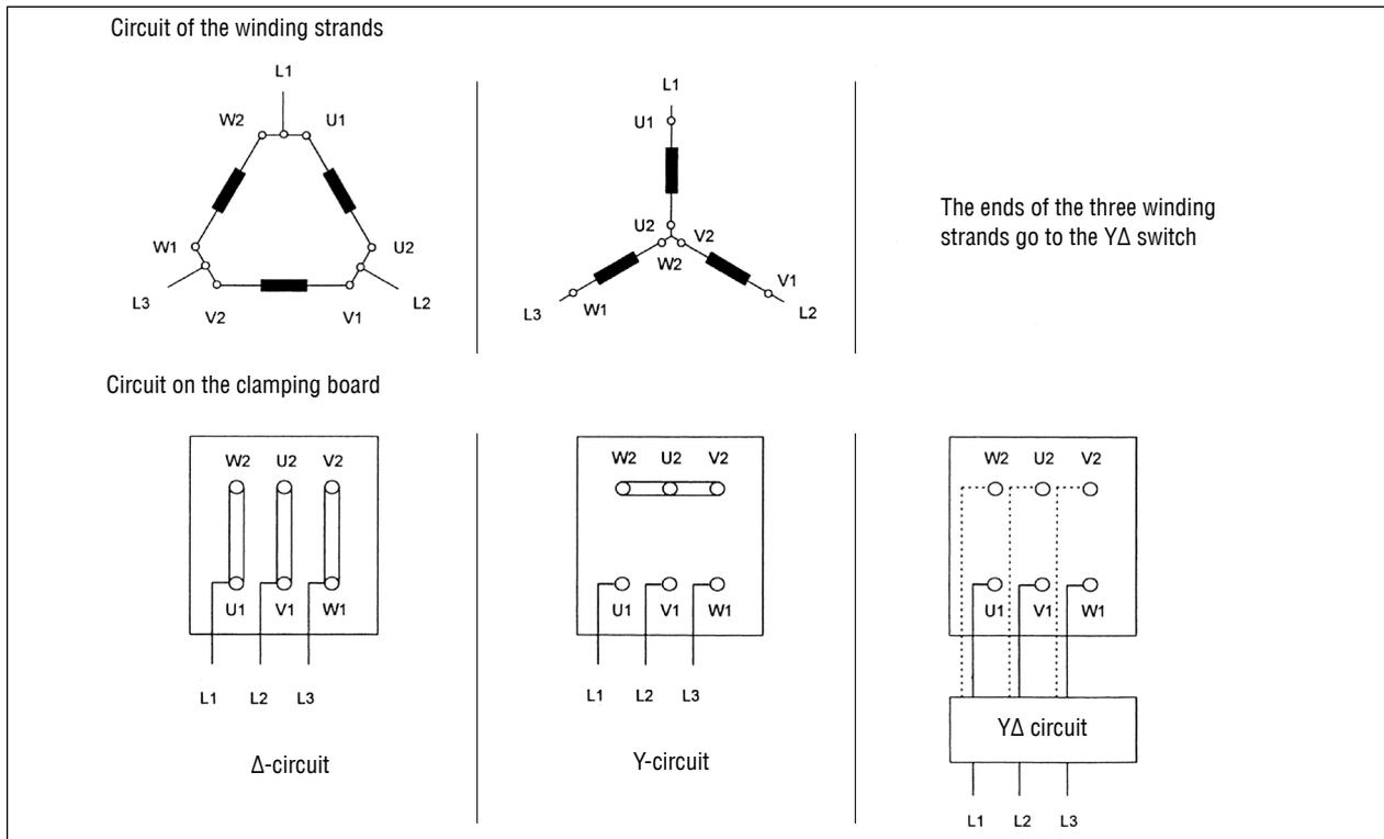
Fig. 47 Circuit of three-phase motors for one speed
