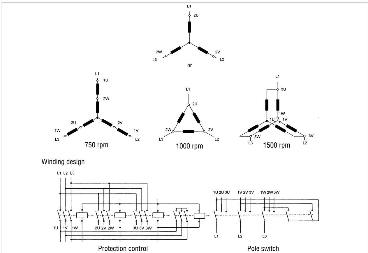
Fig. 50 Circuit of three-phase motors for three speeds
