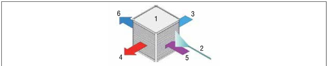
Fig. 56 Cleaning direction for plate heat exchanger
