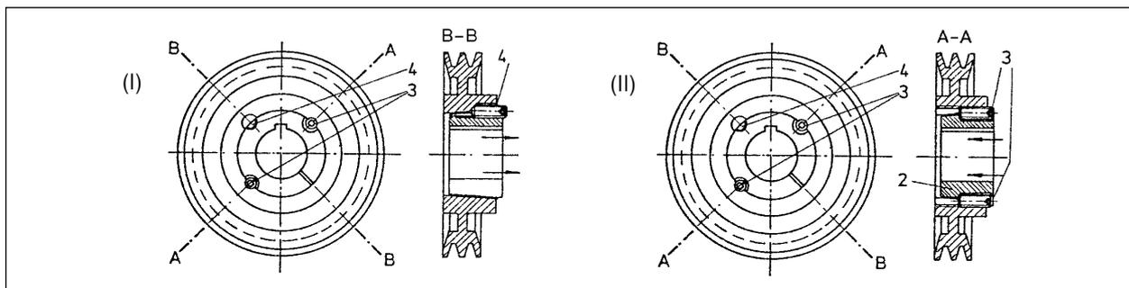
Fig. 61 Fastening of the V-belt pulley
