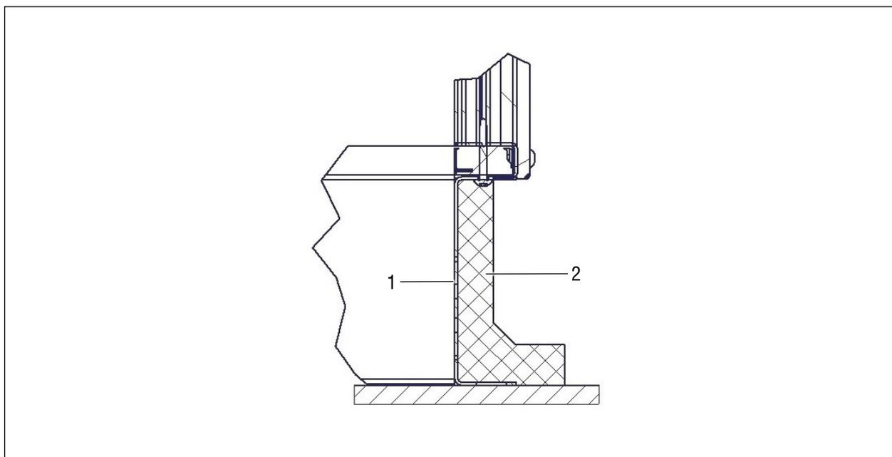
Fig. 21 Factory-mounted base frame
