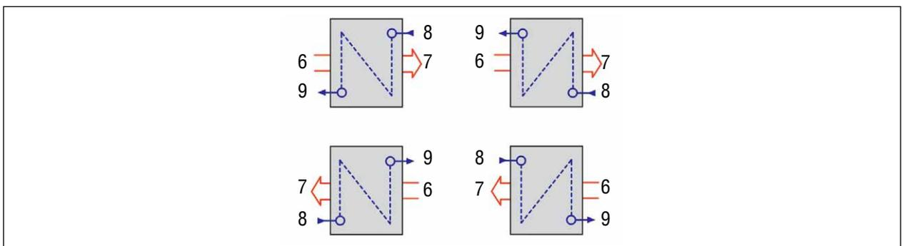
Fig. 39 Counterflow principle for heat exchanger connection
