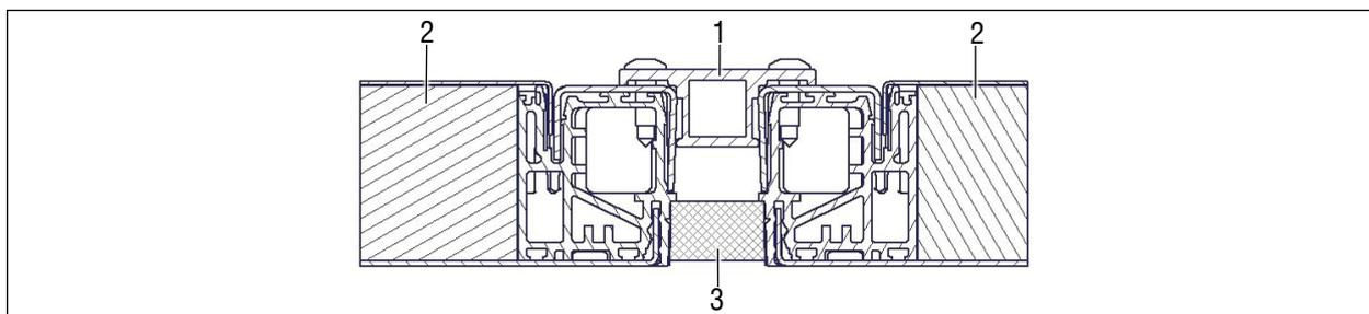
Fig. 17 Unit arrangement next to one another with mixing chamber
