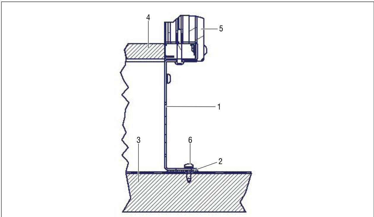
Fig. 13 Unit arrangement one above the other with length offset
