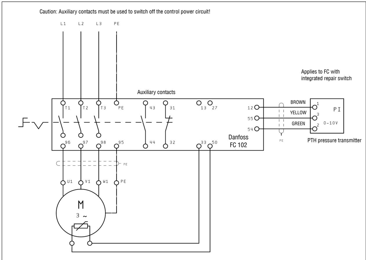
Fig. 52 Circuit of three-phase motors with frequency converter (FC 102) and integrated repair switch.
