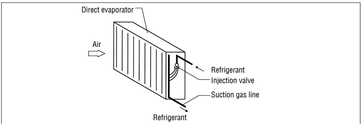
Fig. 43 Air direction when installing a direct evaporator
