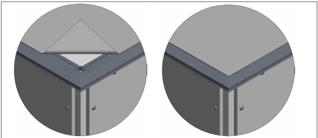
Fig. 27 Weatherproof units with transport device corners on roof assembly with unit frame profile
