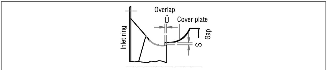
Fig. 67 Gap dimension and overlap
