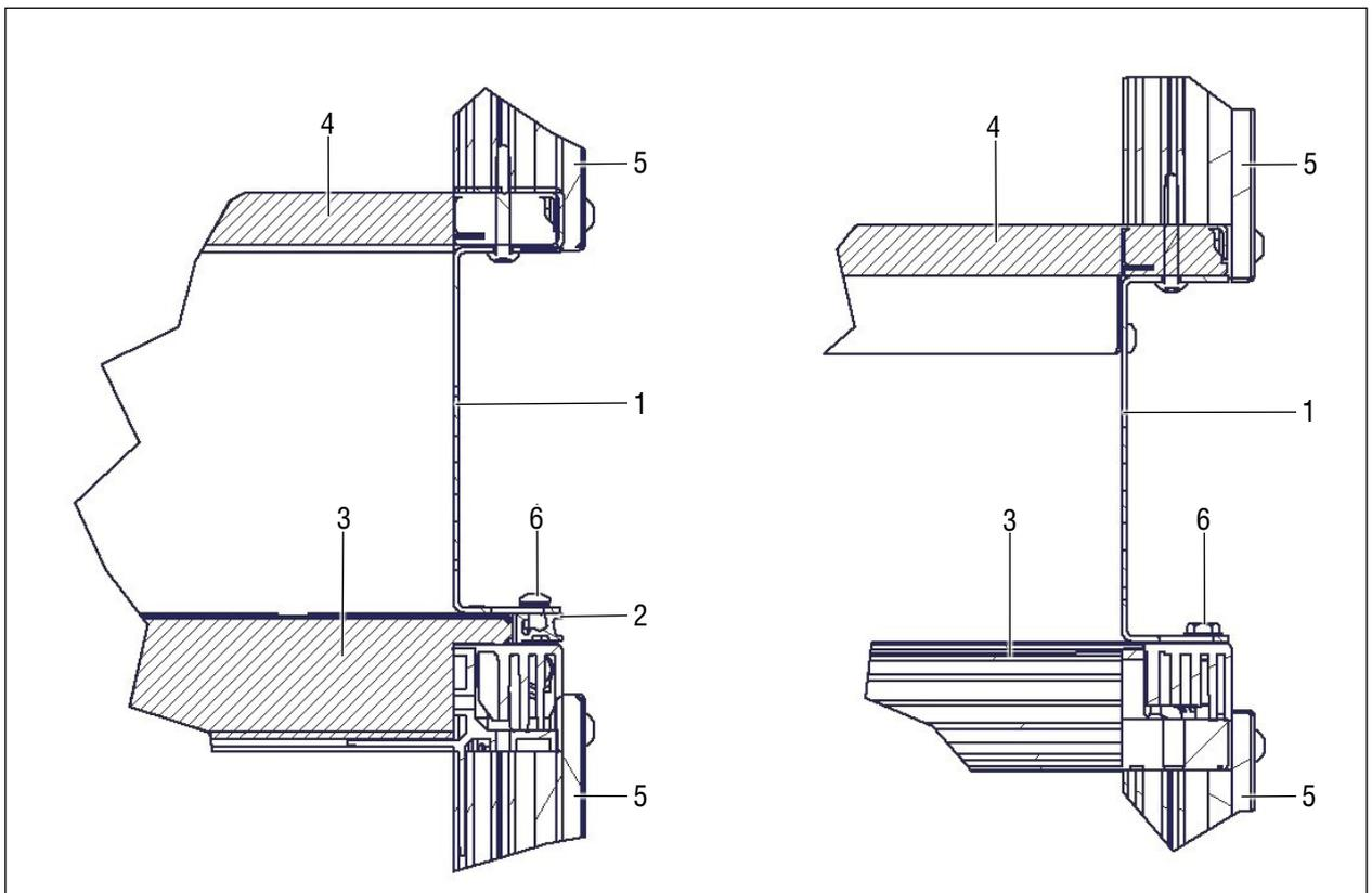
Fig. 10 Unit arrangement roof assembly with unit frame profile (left) and without unit frame profile (right)
