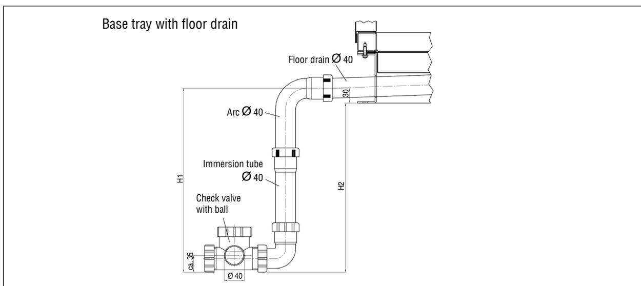
Fig. 46 Connection of the condensate drain with ball siphon with vacuum
