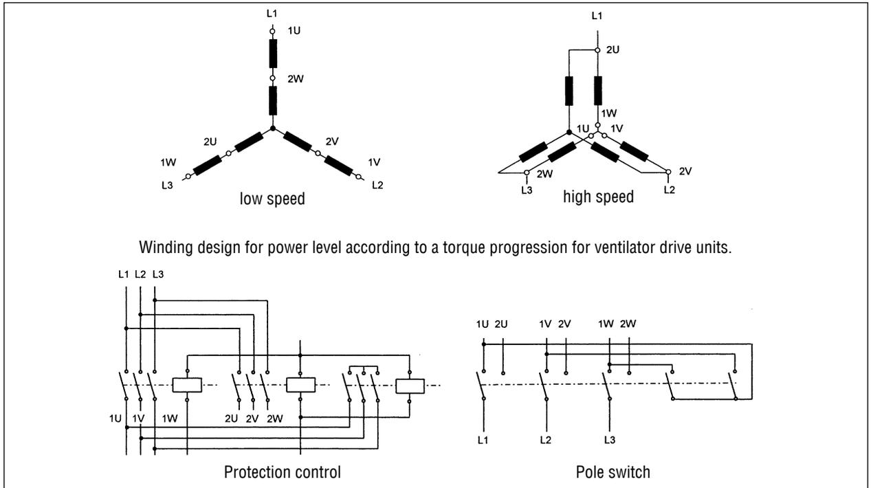
Fig. 48 Circuit of three-phase motors for two speeds in the ratio 1 : 2
