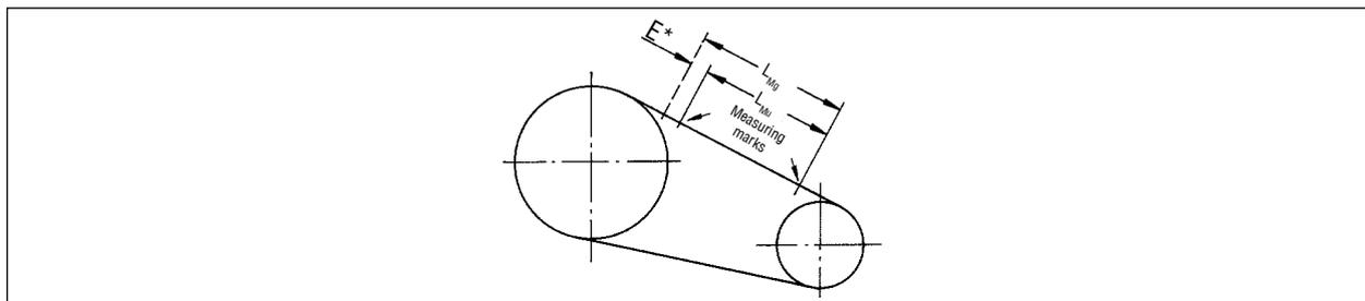
Fig. 60 Checking the belt tension on the flat belt drive
