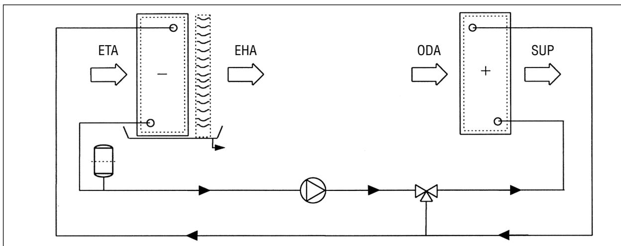
Fig. 42 Schematic diagram of a circulating coil system
