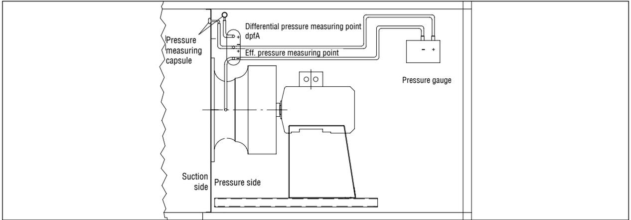
Fig. 65 Air volume determination via measuring differential pressure
