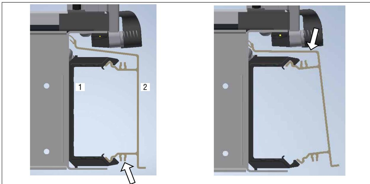
Fig. 33 Disassembly of cable duct cover
