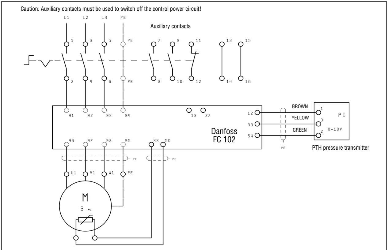
Fig. 51 Circuit of three-phase motors with frequency converter (FC 102) and external repair switch
