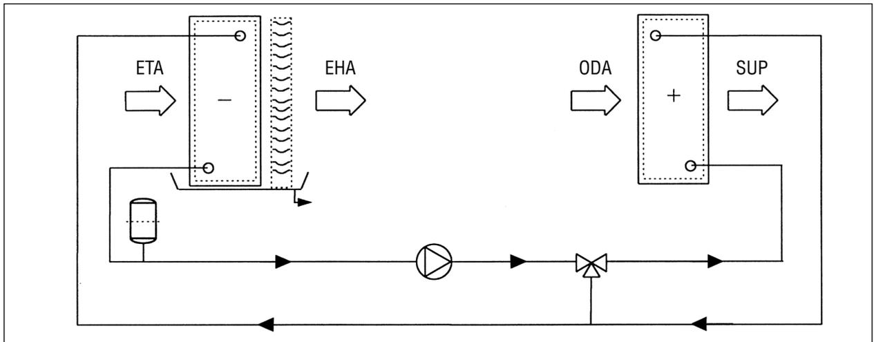
Fig. 54 Schematic diagram of a circulating coil system
