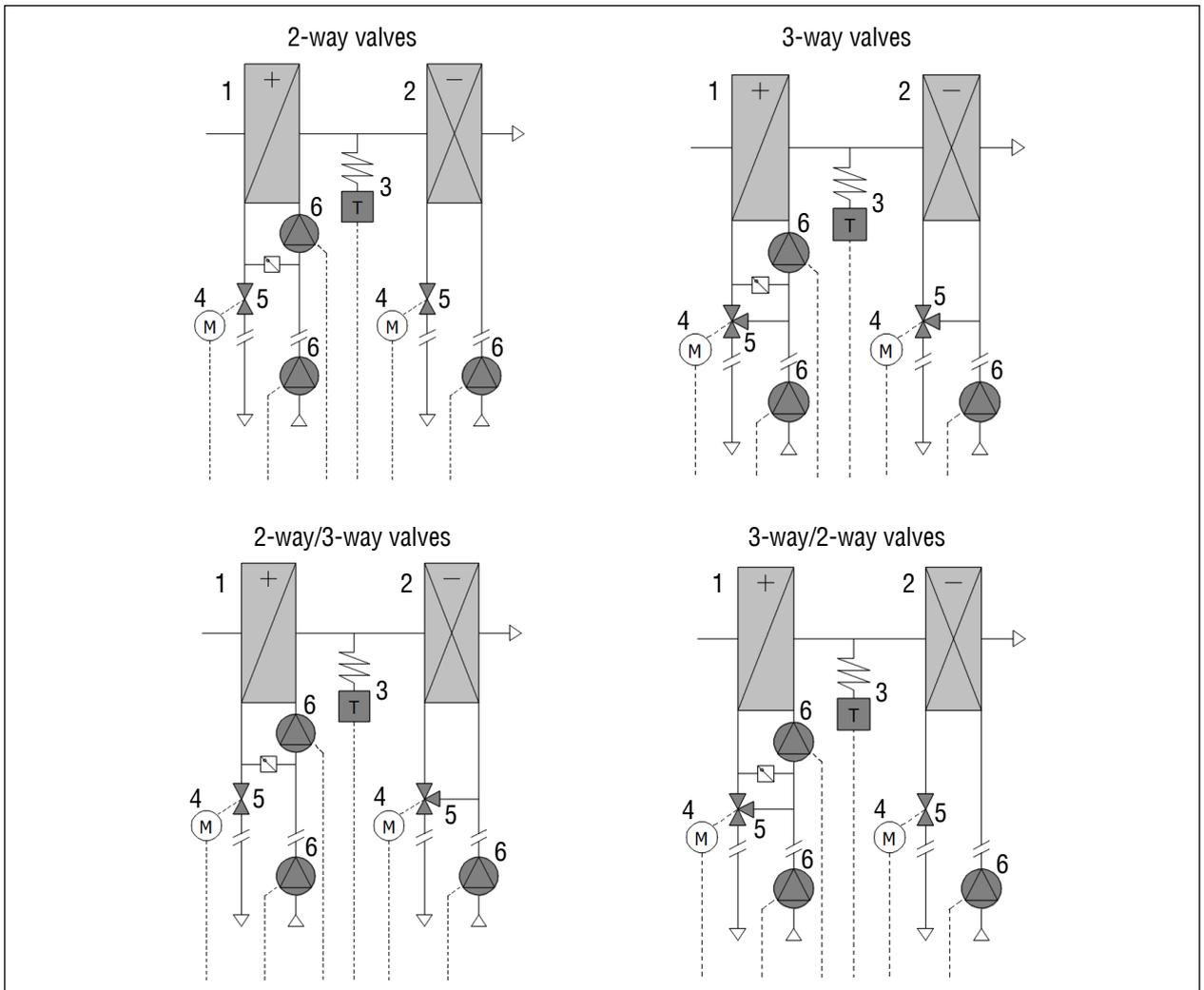
Fig. 38 2-way valve and 3-way valve connection versions
