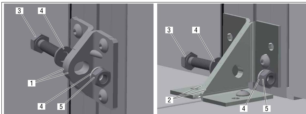
Fig. 9 Unit connections with split housing
