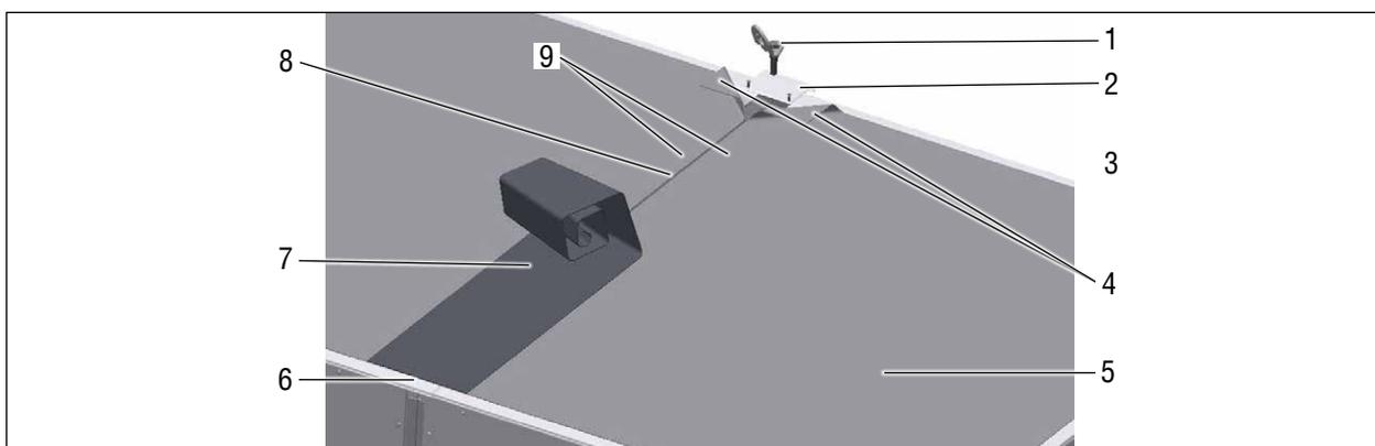
Fig. 24 Sealing of the unit separation points with foil strips
